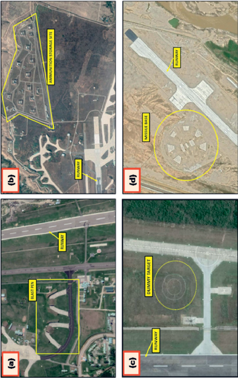
Figure 2: Components of a Military Airport (a) Blast Pen (b) Ammunition Storage Site (c) Dummy Target and (d) Missile Launch Pad near an Airstrip
